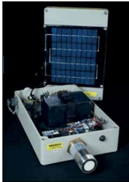
The world's most sophisticated flood monitoring and forecasting system, the US State of Iowa's Flood Centre (IFC), uses more than 200 Senix ToughSonic 30 and ToughSonic 50 ultrasonic sensors to measure water levels in streams across the state.
